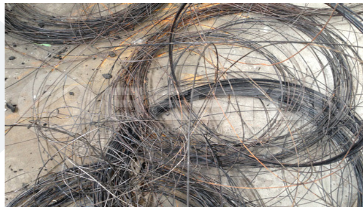
Steel bars after being withdrawn from the tires
